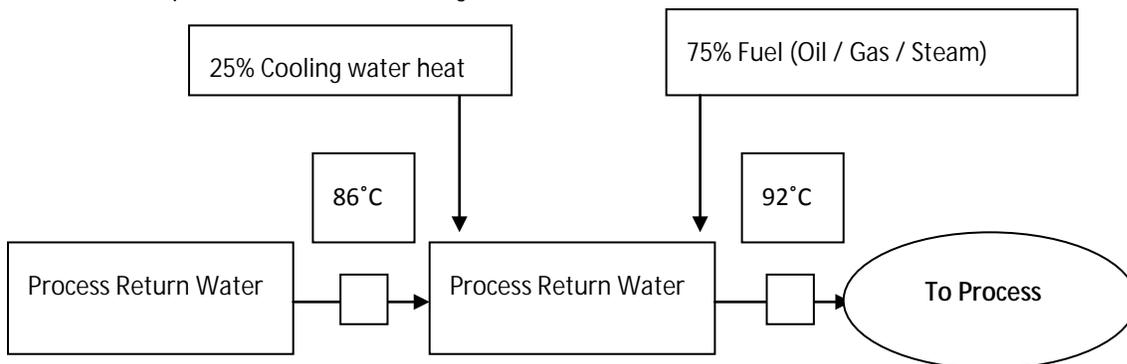
Figure 3: Illustration of energy efficiency through use of Heat Pump
